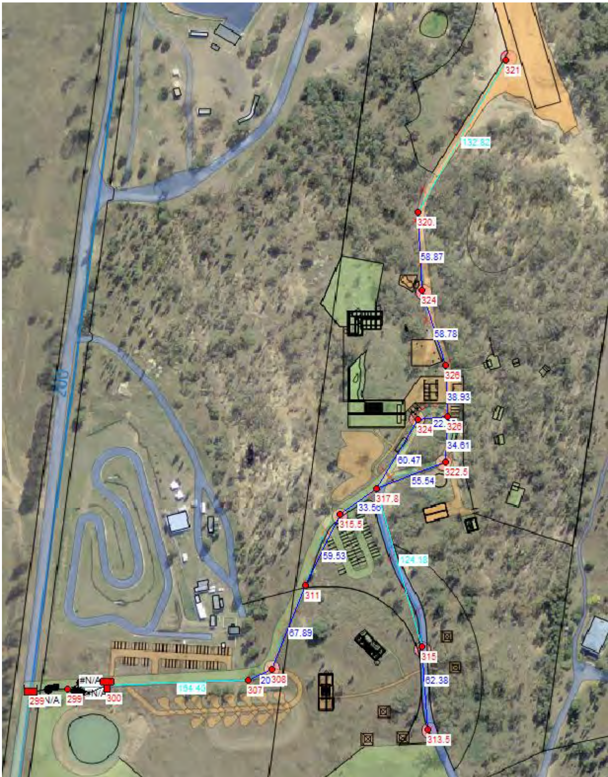
Model layout with pipe lengths (m) and junction elevations (m AHD)
