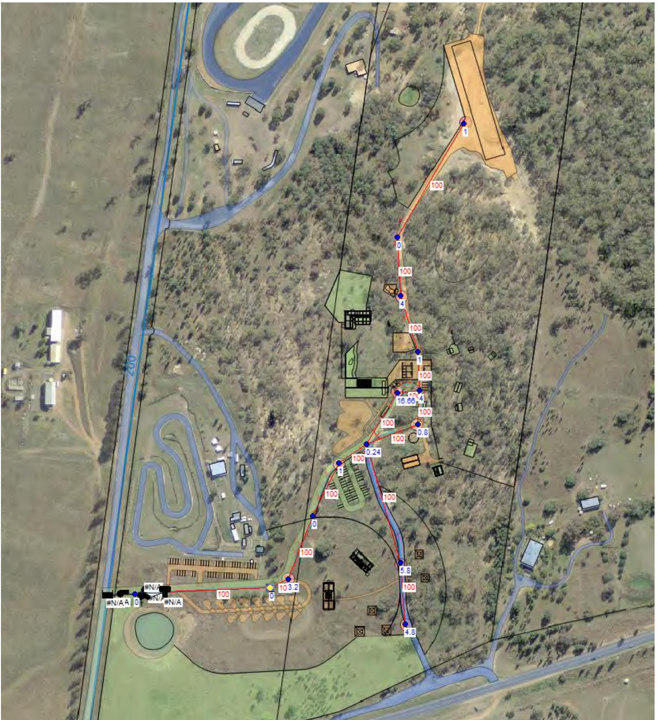
Model layout with pipe diameters (mm) and demands at junctions (ET)
